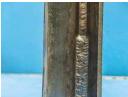
Multi pass welding - vertical up
