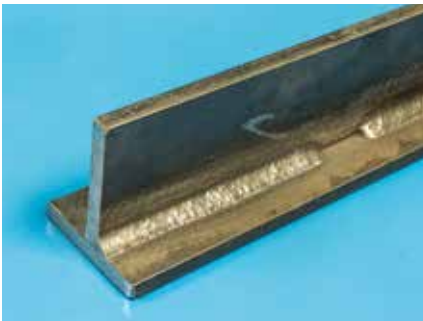
Clean weld surface
