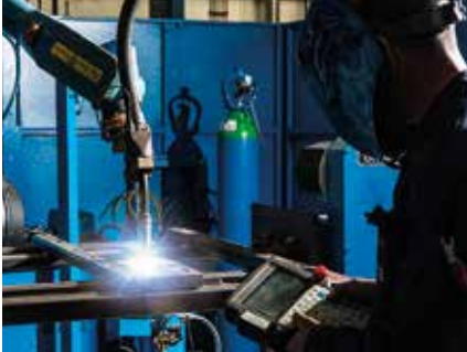
Robotic MAG welding
