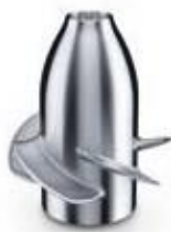
Fan Wheel Material: Stainless steel Laser Deposition Welding: 312 min. Milling: 240 min. Dimensions: Ø 160 mm × 160 mm
