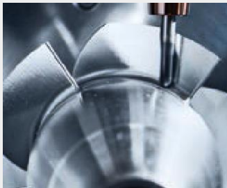
6: Finish milling the vanes
