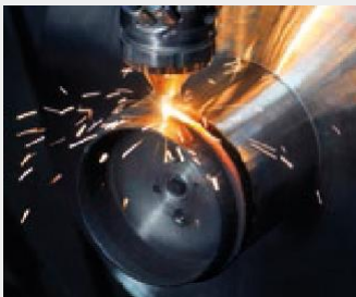
2: 90° swivel: Generation of the flange
