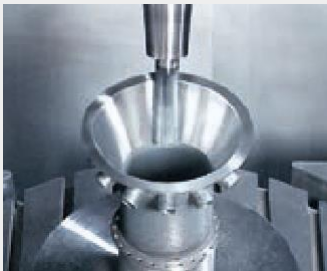
6: Finishing of the inner and outer contour
