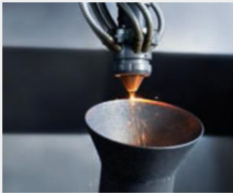
4: Continuation of the cylinder generation with conical funnel
