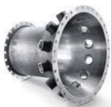
Turbine casing Material: Stainless steel Laser Deposition Welding: 230 min. Milling: 76 min. Dimensions: Ø 180 mm × 150 mm
