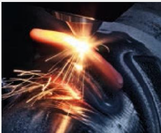
5: Building the vanes on the cylinder
