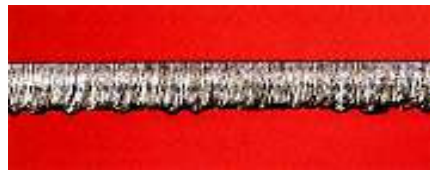
Test on 4 mm thickness Carbon Steel Controlled impurities are: moisture (H 2 O) ≤ 10 ppm Argon (Ar) ≤ 500 ppm
