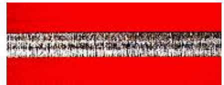
Test on 4 mm thickness Carbon Steel Controlled impurities are: moisture (H 2 O) ≤ 10 ppm Argon (Ar) ≤ 500 ppm
